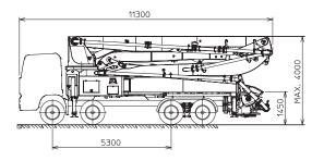
Dimensions varying according to truck assembly
